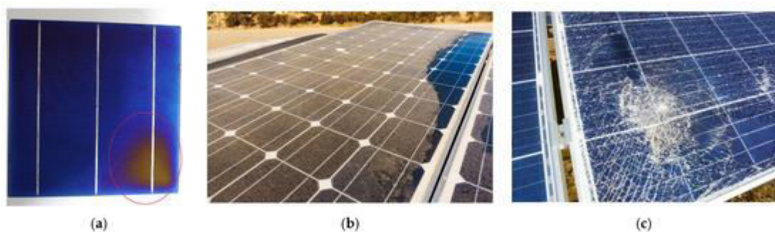
Figure 1. (a) Defective, (b) dusty panel, (c) physical damage.
